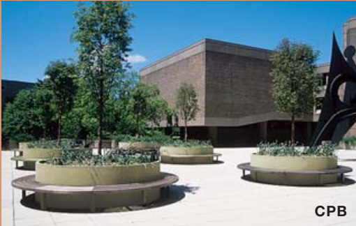
Standard widths: 18"; circular/square planter benches overall d or l 7'-11' Rect. planter benches: overall 48" l min. and 48" w -single, 66" w -double.
