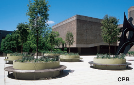
Standard widths: 18"; circular/square planter benches overall d or l 7'-11' Rect. planter benches: overall 48" / min. and 48"w-single, 66"w-double.
